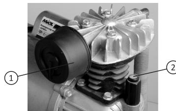
**Fig. 3. Installation of air filter**
